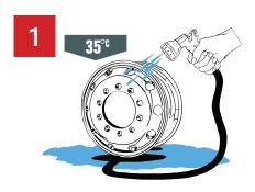
Allow the wheels to cool below 35°C, then remove the nut covers. Rinse with clean water to avoid scratches and corrosion, and ideally, use a high-pressure washer.
