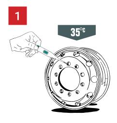
Make sure you allow the wheels to cool below 35°C, then remove the nut covers.
