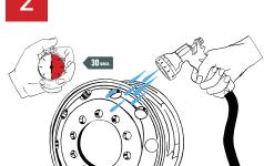
In order to avoid scratches and corrosion, the wheels should be washed with clean water.
